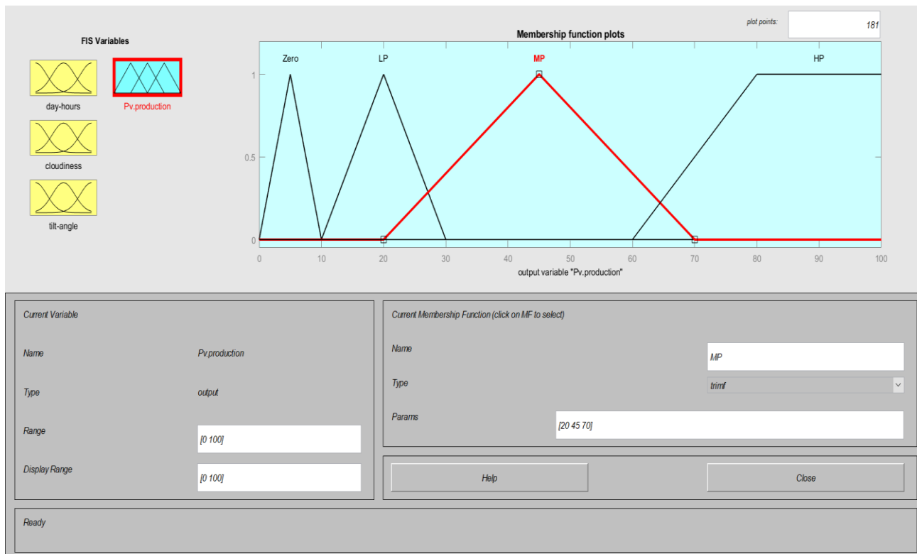
Fig. 8. Membership functions indicator PV production output
