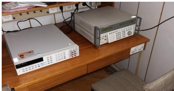
Fig. 14. The LEM primary and secondary reference standards for electrical quantities, Agilent 3458A and FLUKE 5500A
