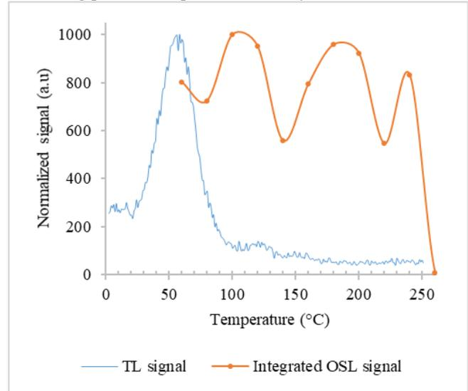
**Fig. 6.** Comparison of preheating temperature dependence of OSL response with TL glow curve
