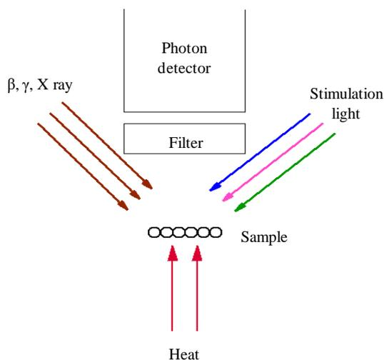
Fig. 1. Schematic diagram of the Riso TL/OSL reader
