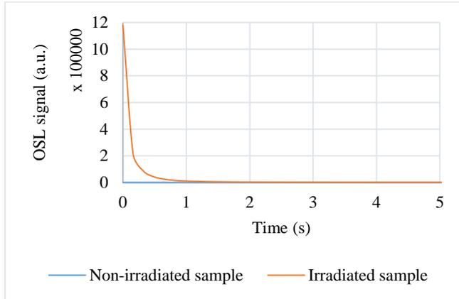
**Fig. 4.** OSL signals of non-irradiated sample and irradiated sample (300 mGy)
