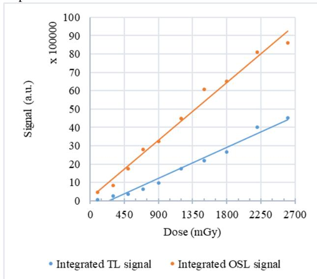
**Fig. 5.** Dependence of the luminescence signal on the dose
