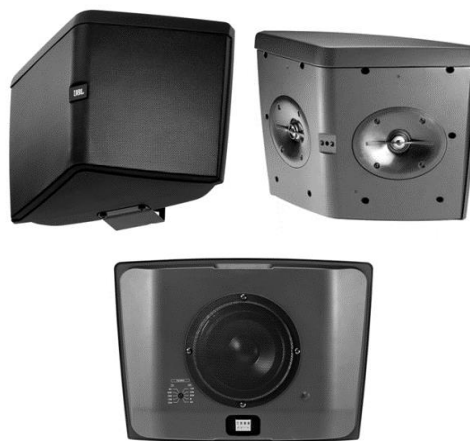
Fig. 9. Commercial loudspeaker (JBL Control HST) with mid-bass unit positioned toward the wall at close distance, plus two tweeters in short horns, positioned outwards
