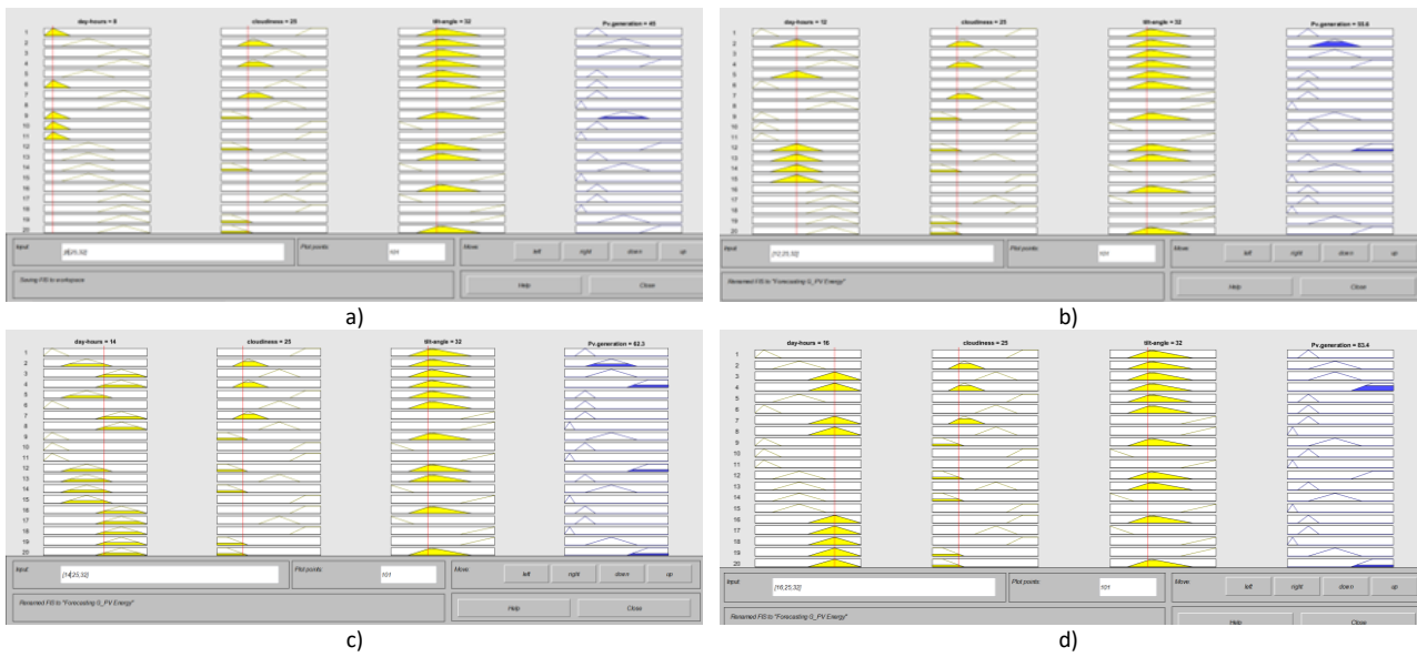
Fig. 11. The influence of the input hours of the day on the value of the output PV production on fuzzy inference rules a) “hour of the day” is 8 and all other inputs are constant; b) “hour of the day” is 12 and all other inputs are constant, c) “hour of the day” is 14 and all other inputs are constant; d) “hour of the day” is 16 and all other inputs are constant
